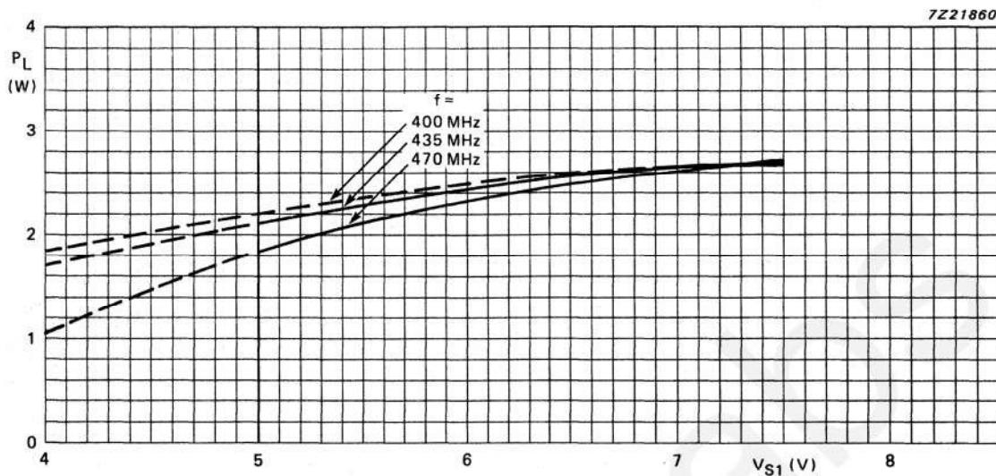
Fig.5 Load power as a function of  $V_{S1}$ ;  $V_{S2} = 7.5$  V;  $P_D = 50$  mW; typical values.
