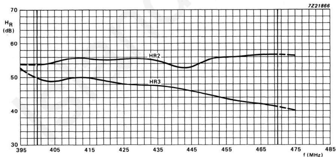
Fig.10 Second and third harmonic distortions as functions of frequency;  $V_{S1} = V_{S2} = 9.6$  V;
