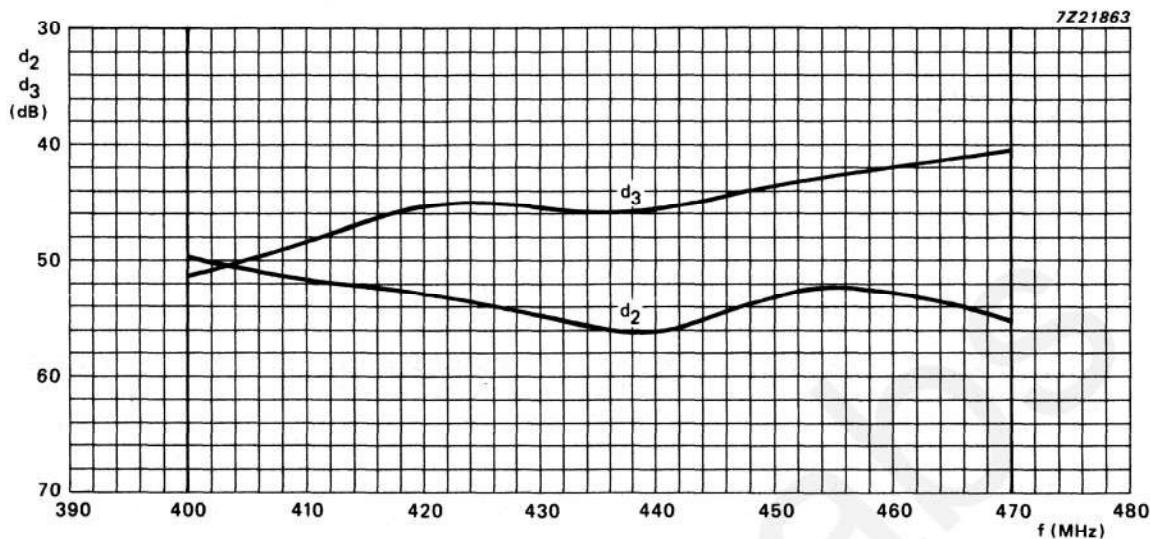
Fig.9 Second and third harmonic distortions as functions of frequency;  $V_{S1} = V_{S2} = 7.5$  V;
