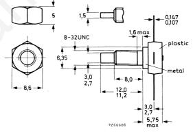
Torque on nut: min. 7.5 kg cm (0.75 Newton metres) max. 8.5 kg cm (0.85 Newton metres) Diameter of clearance hole in heatsink: max. 4.17 mm.
