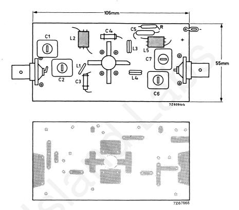
The circuit and the components are situated on one side of the epoxy fibre-glass board, the other side being fully metallised to serve as earth. Earth connections are made by means of hollow rivets.
