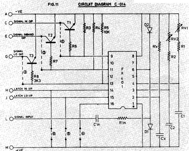
FIG.12 OVERSPEED ALARM WITH LATCHED OUTPUT
