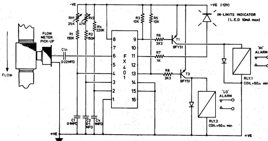
Fig.14 shows how the FX-401 is used to obtain comprehensive monitoring of a flowrate. When signals from the flow transducer lie between f1 and f2 (90Hz and 80Hz), the IN-LIMITS L.E.D. is illuminated. If the signal rises above f1 the HI alarm relay operates, if it falls below f2 the LO relay is turned ON. Only one output is energised at any time and the set-point thresholds are very sharp (0.1% differential typical).
