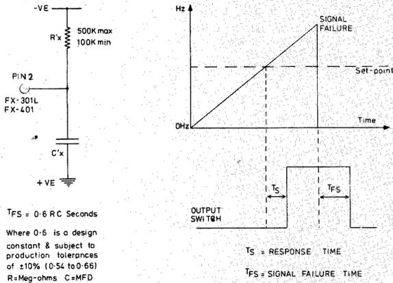
For general purpose applications a convenient value for T<sub>FS</sub> is  $\frac{10}{f_2 \text{ (Hz)}}$
