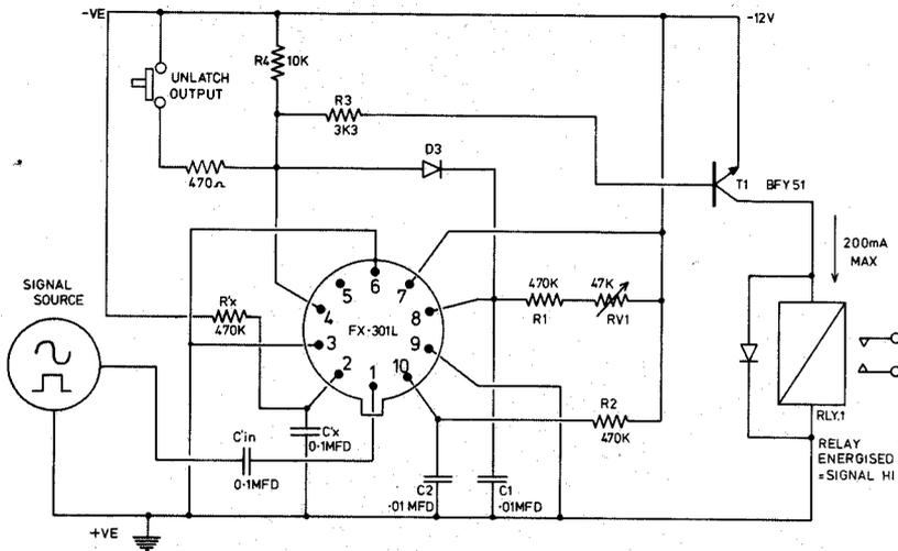
Fig.12 illustrates a typical overspeed alarm circuit using FX-301L. When the input frequency exceeds set-point f1, the relay is latched ON. The relay may be reset, or unlatched, by closing the push-button contacts.
