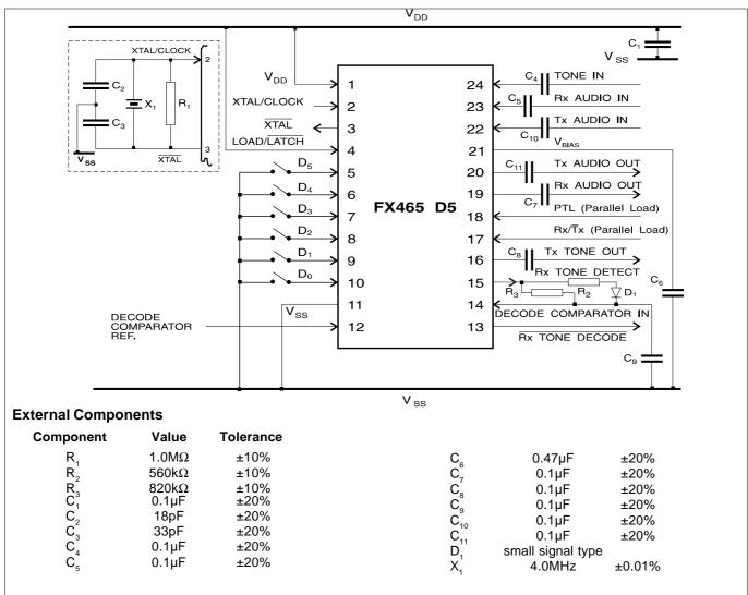
**Note:** The values specified for  $R_1$ ,  $C_2$  and  $C_3$  have been found to be satisfactory when used with a crystal ( $X_1$ ) whose equivalent series resistance is <= 1000 ohms. The crystal manufacturer should be consulted to determine optimum values for different crystals.
