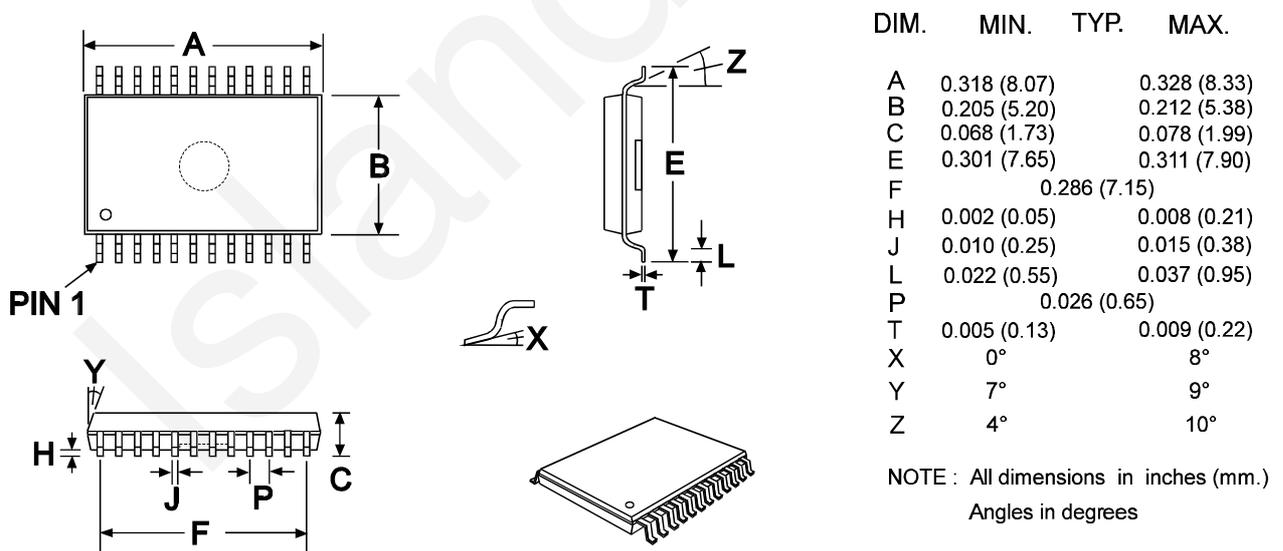
Figure 23 D5 Mechanical Outline: Order as part no. FX909AD5
