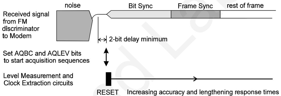
Figure 16 Bit Clock and Level Acquisition Example
