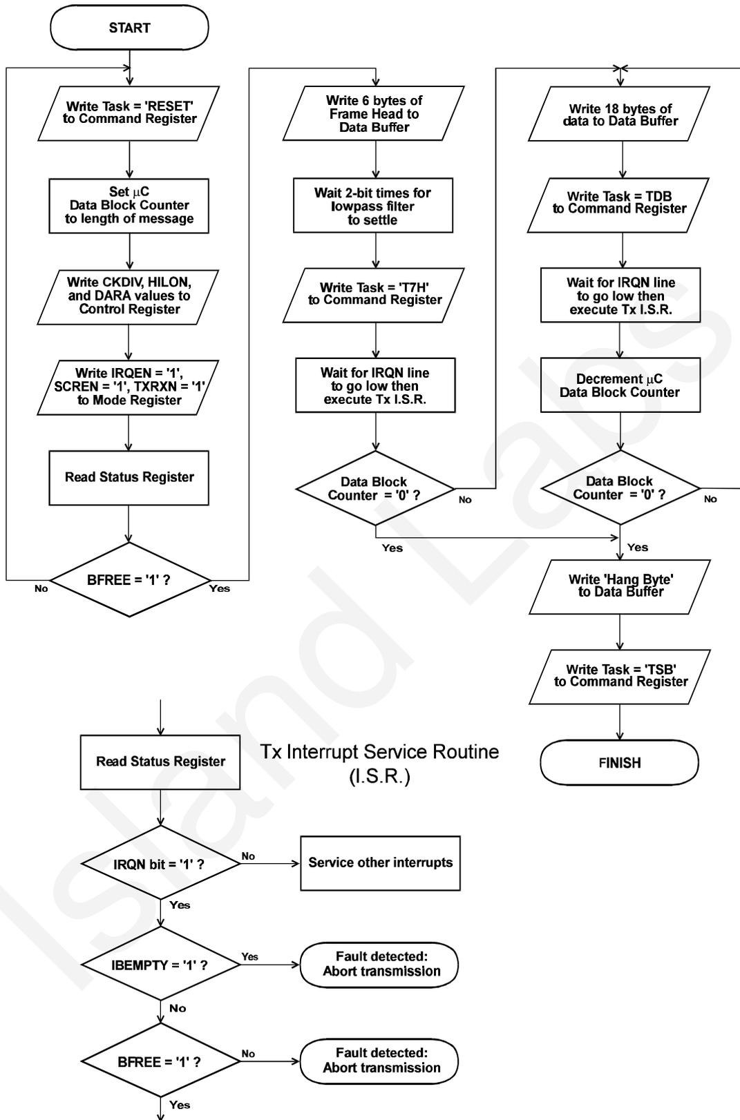
Figure 14 Transmit Process
