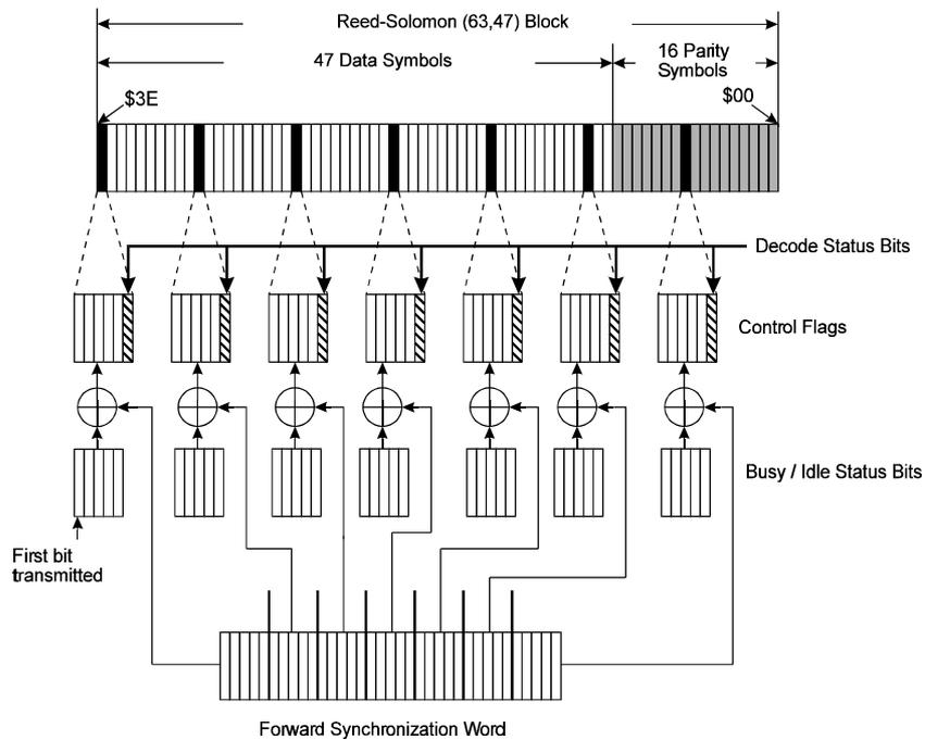
Figure 6 Forward Channel Transmission Structure
