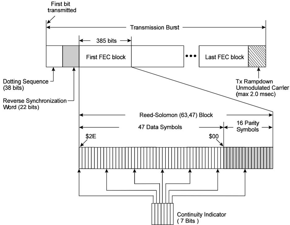
Figure 5 Reverse Channel Transmission Structure
