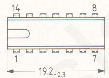
Plastic plug-in package 20 A 14 DIN 41866 14 pins, dual-in-line Weight approx. 1.1 g
